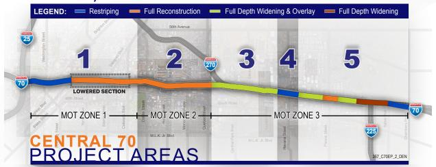
**MOT Zone 1** starts east of I-25 and includes all of Area 1 with work limits extending to just east of Colorado Boulevard. Area 1 is focused on the construction of the Lowered Section and is divided into two phases requiring only one traffic shift for both WB and EB I-70.
